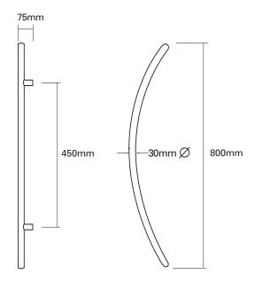
Glass drilling: 2 x 16mm Ø holes A gently curved handle which can be fitted at 45° across the door.
