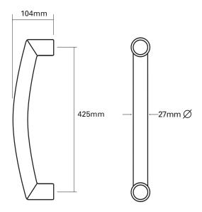
Glass drilling: 2 x 16mm Ø holes A modern, simple design of handle which looks superb in the satin finish.
