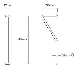
Glass drilling: 2 x 10mm Ø holes A contemporary design, often specified for double doors. They can be supplied as a single handle and are manufactured from high grade marine stainless steel.
