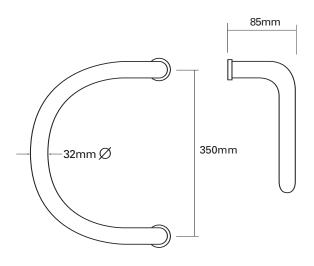
Glass drilling: 2 x 16mm Ø holes This curved handle offers a really impressive appearance particularly in the polished finish.
