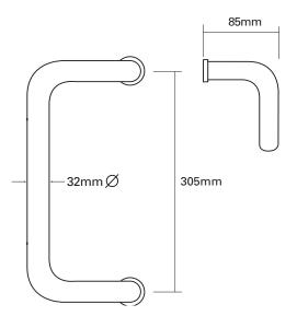
Glass drilling: 2 x 16mm Ø holes A popular two bend design of handle which is specified mainly for retail installations.
