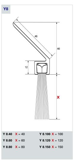
Picture 1 Brush profile H used on cable ducting
