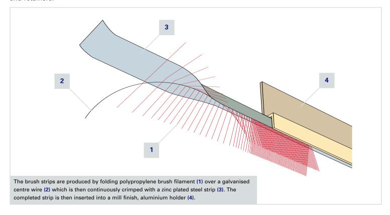
All strips are 3m long with various brush lengths and the aluminium holders are available in 3 profiles; **F, Y** and **H**.
